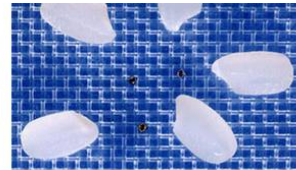
A New RFID with Embedded Antenna \mu -Chip
