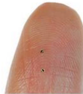
A New RFID with Embedded Antenna \mu -Chip
